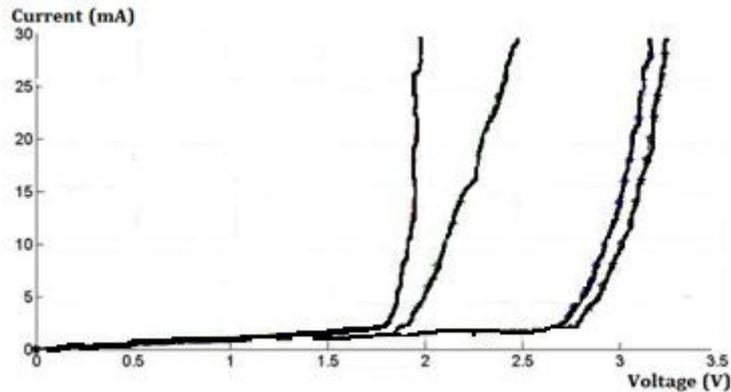
**Figure 1.** Current-voltage characteristic of the LED lighting system.
