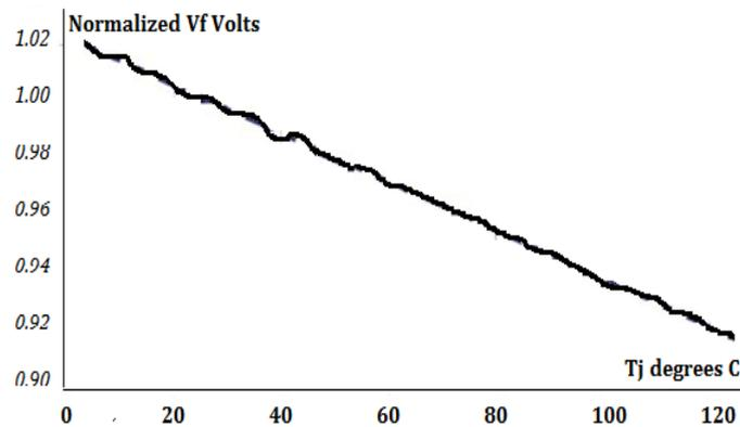
**Figure 2.** Change in voltage due to heat in the LED lighting
